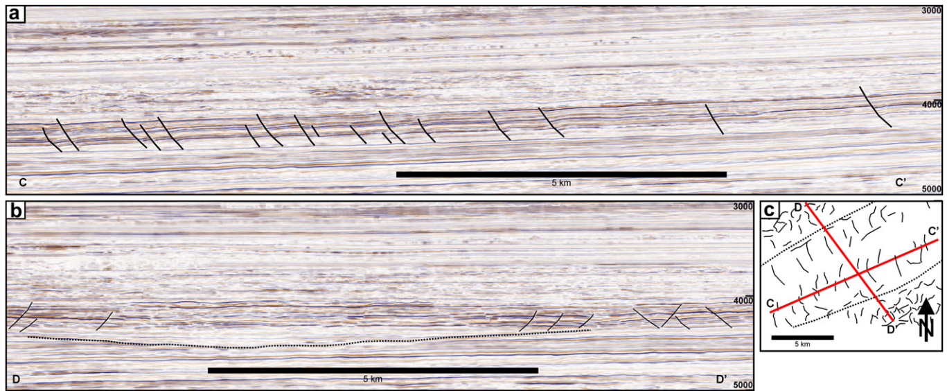
Fig. 9. Representative seismic sections from Canyon II (a) along the axis of the canyon, showing a domino array of antithetic faults, and (b) perpendicular to the canyon axis. (c) Fault trace map showing the two dominant fault trends above the canyon. Canyon base and margins are marked by dotted lines. Vertical scale in (a) and (b) is two-way time in milliseconds.
